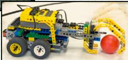
Gear up rotation sensor to increase precision
