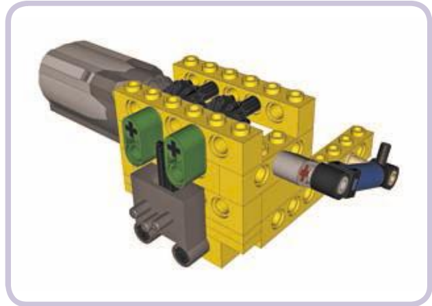
Figure 10-11: An autovalve uses a sliding worm gear to control a compressor and a pneumatic valve with just one motor.
