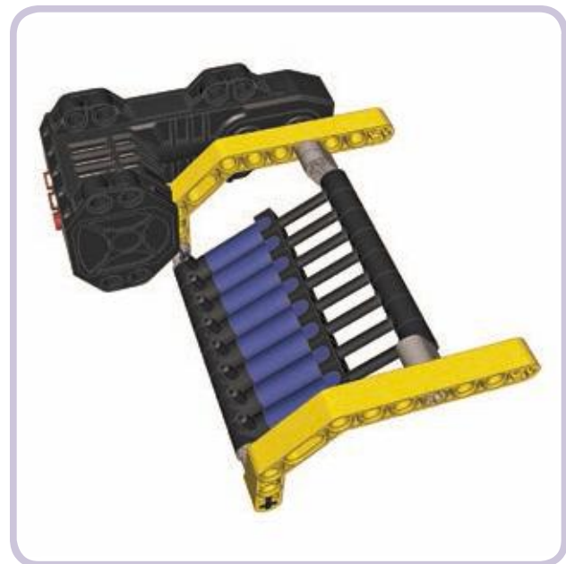
Figure 10-1: An eight-pump compressor driven by the RC motor. This design is a real monstrosity in the world of LEGO compressors.
