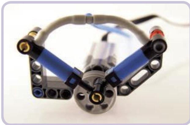
Figure 10-2: A compressor with two pumps that work alternately, both attached to two wedge belt wheels. The design is small, but it's difficult to add more pumps to it. In this compressor, the pumps are 90 degrees out of phase rather than 180 degrees, so the pressure is still "uneven." In other words, one pump is not fully extended while the other is fully compressed.
