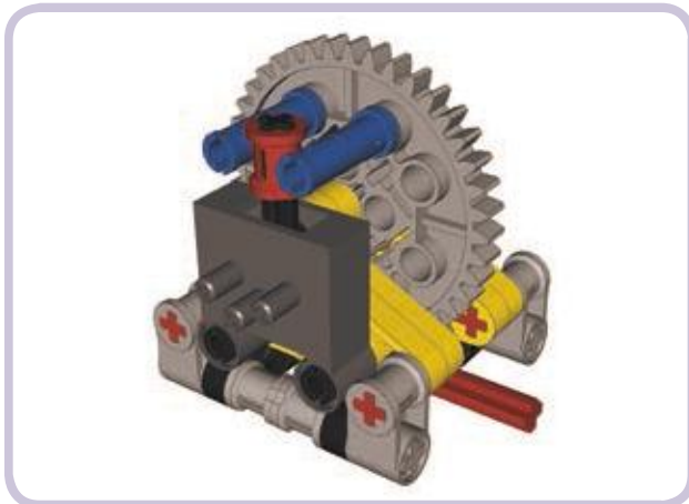
Figure 10-10: This high-precision valve-switching mechanism makes use of a worm gear and a 40-tooth gear to ensure accuracy. The red bush on the valve's lever improves it further by reducing backlash. Note that there is no safety clutch in this assembly; because the mechanism multiplies the motor's torque by a factor of 40, there is a chance that some pieces may be damaged if the motor doesn't stop at the right moment. To lessen this risk, a clutch can be added between the valve and the motor.
