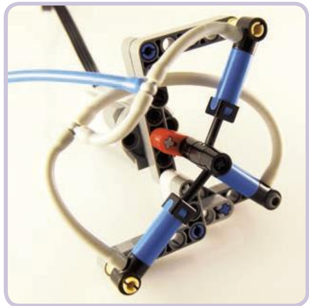
Figure 10-4: It's perfectly possible to split pumps in a compressor into three groups.
