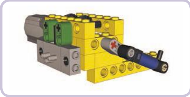
Figure 10-12: An autovalve can be created with both types of pneumatic valves (the older one is shown here) and with any compressor whatsoever—the single-pump compressor here is just an example.
