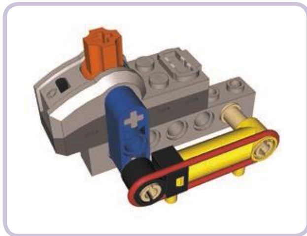
Figure 10-13: A close-up view of a pressure switch. The switch usually needs adjusting to activate at the desired pressure threshold. It can be fine-tuned by adjusting the rubber band's strength, the angle of the cylinder relative to the lever, and the length of the lever. It is also possible to use old 9V switches, which offer less resistance, or to use multiple cylinders. Large cylinders can be used as well, although their large capacity makes them less sensitive and therefore less useful in system that must react to small changes in air pressure.
