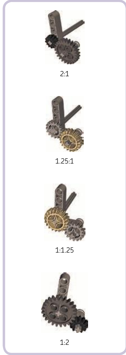
Figure 10-7: The four gear combinations suitable for the rocking compressor, with their ratios labeled
