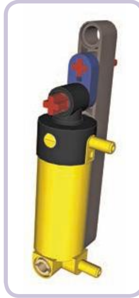
Figure 10-15: A simple way to connect the cylinder to a shaft is to use a cam made of a short beam. However, a cylinder can extend by 4 studs, but here it's allowed to extend by only 3.
