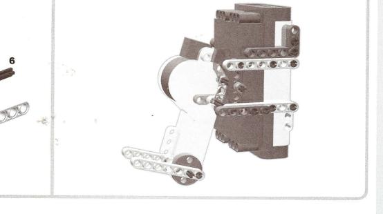
e beam is held on with both an axle and a pin.
