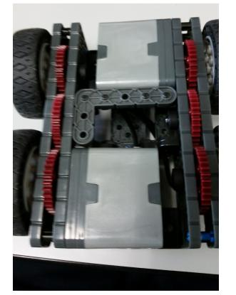
Make sure the motor is secure and attach the other side.
