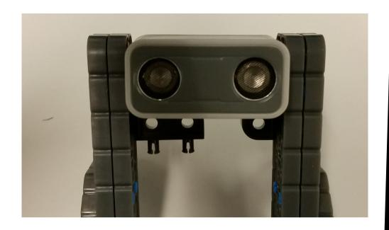
Attach the ping and touch sensors as shown.
