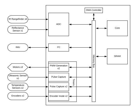
Fig. 1. Example of a RCJ Rescue Maze robot architecture utilizing hardware peripherals of a microcontroller
